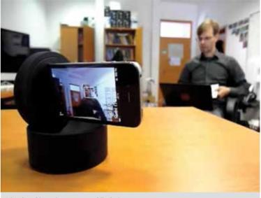
Visual tracking using a smart mobile device
