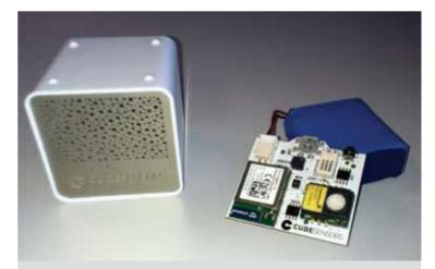
We have developed a firmware for the Cubesensors devices that monitor the living conditions in a home or an office. It features monitoring of air quality, temperature, humidity, pressure, noise, illumination, and shaking.
