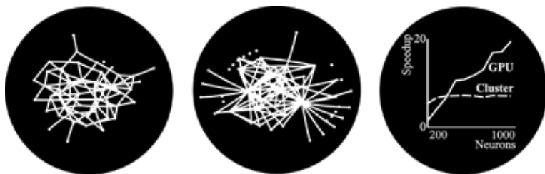
Graphs of initial (left) and trained (center) fully recurrent neural network and speedups achieved on parallel architectures with respect to a standalone computer (right)
