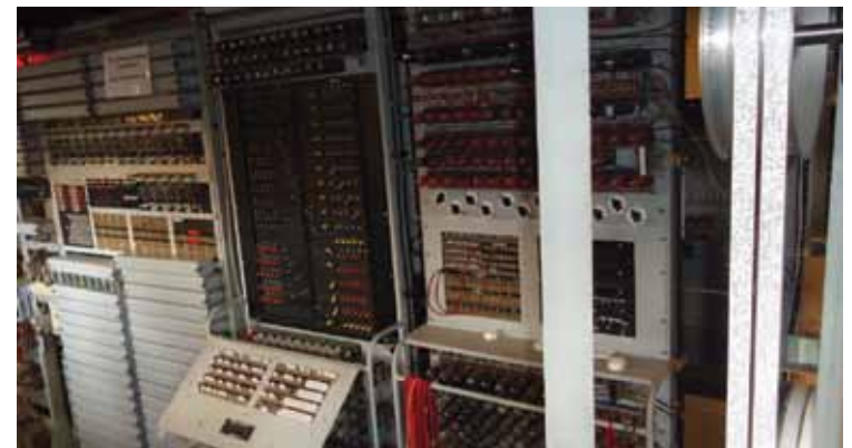
Colossus was the first electronic computer, used by British codebreakers during World War II for cryptanalysis of the Lorenz cipher
