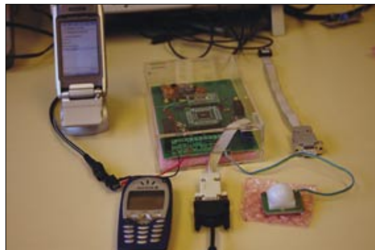
Lab-Architecture and Signal Processing-picture.JPG): GSM module for remote control system
